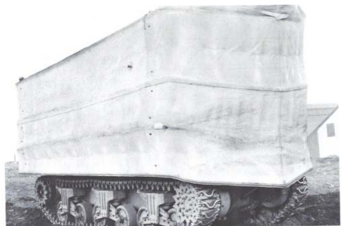
The screens took 15 minutes to inflate, and rose to a height of 7 feet. When the bracing struts were broken, the screen would fold like a concertina. [Photo courtesy of IWM]
