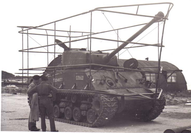
A DD Sherman Tank fitted with the tubular support rails and bracing struts. The inflatable rubber support tubes have yet to be fitted.
